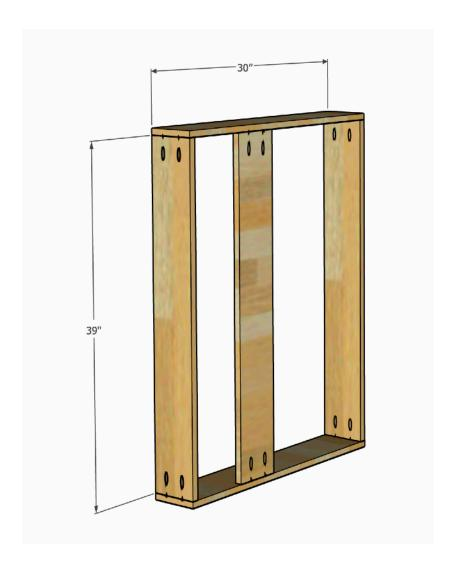
Once both sides are built, attach the front and back runner. When you drill the pocket holes on the runners, be sure to off set them so they don't hit the screws coming from the center board on the armrest, since they are going into the same board. These should line up with the side supports at 10" from the bottom/ ground.
